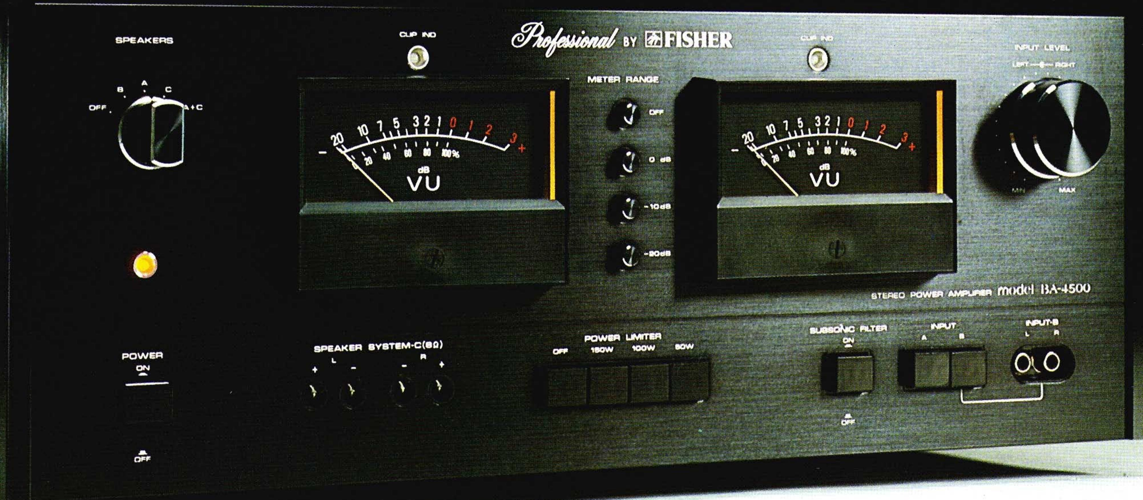
All stages pure complementary symmetrical SEPP OCL circuitry delivers a full 300W RMS output power at 8 ohms, both channels driven from 20 to 20,000Hz with only 0.02% T.H.D. This advanced circuitry suppresses noise so completely that the S/N ratio of this unit is an amazing 105dB. The super-high 60V/ $\mu$ s slew rate also ensures superior handling of rapid signal changes, thereby suppressing transient intermodulation distortion.
